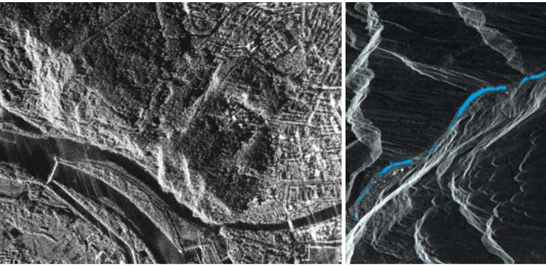
COSMO-SkyMed 2 StripMap HIMAGE acquisition (3 m resolution) over the city of Guan Xian in China and the Zipingpu dam, acquired on 13 May 2008, the day after the terrible earthquake hit this region. In detail, an image of the area of Beichuan, where large landslides blocked rivers and roads, acquired the following day by COSMO-SkyMed 1 satellite in Spotlight-2 mode.
